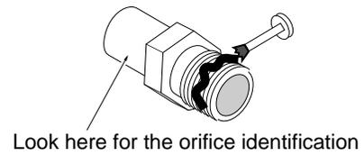
(d) Screw the LP orifice until orifice protrudes 15/16" (23.8mm) indicating full insertion (use wrench to secure manifold when re-attaching orifice).
