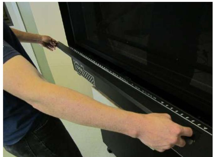
2. Remove the three screws holding the screen in place (1/4" nutdriver- magnetic driver recommended). Then pivot the screen down slightly until the clips on the bottom disengage from the glass frame.
